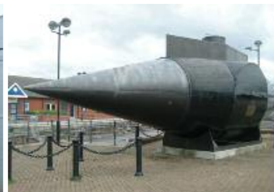
Left: Depth-charge damage that sunk German submarine U-534. Right: This is a full-size reconstruction of one of the first submarines ever built. Designed by Birkenhead curate the Rev George Garrett, the iron and wood vessel was built in 1879 and was the first to be successfully propelled mechanically underwater. Manned by a crew of three, and named Resurgam - Latin for 'I shall rise again' - it sank in a storm off North Wales in 1880
