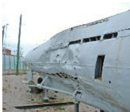
Left: Depth-charge damage that sunk German submarine U-534. Right: This is a full-size reconstruction of one of the first submarines ever built. Designed by Birkenhead curate the Rev George Garrett, the iron and wood vessel was built in 1879 and was the first to be successfully propelled mechanically underwater. Manned by a crew of three, and named Resurgam - Latin for 'I shall rise again' - it sank in a storm off North Wales in 1880
